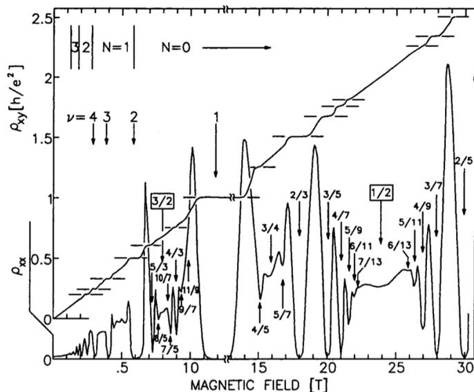
**Figure 1.4:** Fractional quantum Hall landscape: the Hall resistivity exhibits plateaux at integer and fractional values of the von Klitzing constant  $h/e^2$ . In particular only odd denominators plateaux are observed at fractional fillings in the two lowest Landau levels. Nowadays more than fifty plateaux are observed only in the lowest Landau level.
