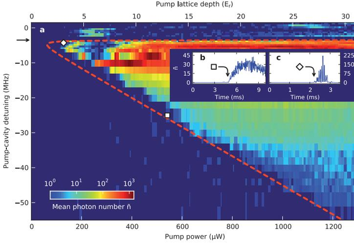
**Figure 3.2:** Experimental phase diagram: the mean intracavity photon number is displayed as a function of the pump power and of the pump-cavity detuning. Every pixel depicted in the plot is a single experiment run with different parameters. This result is in good agreement with the theoretical prediction of the Dicke model (red dashed curve).
