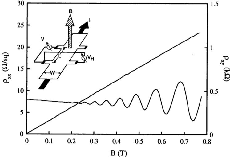
**Figure 6.1:** Classic Hall effect: low temperature and moderately low  $B$ . The insert shows the measurement geometry. The voltages  $V_x$  and  $V_y$  are respectively measured in the two perpendicular directions on the sample.  $\rho_{xx}$  is the resistivity across the square.  $\rho_{xy} = V_y/I$  is the Hall resistivity. Image taken from [114].
