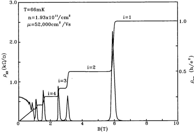
**Figure 6.2:** The integer QH effect (IQHE). In a classical electron gas the Hall resistivity  $\rho_{yx}$  is proportional to the magnetic field  $B_{\perp}$ . However, the Hall resistivity  $\rho_{xy}$  shows a stair case in an actual sample, with the plateau crossing the classical line at  $\nu = 1, 2, 3, \dots$ . The diagonal resistivity  $\rho_{xx}$  vanishing at these points. Image taken from [114].
