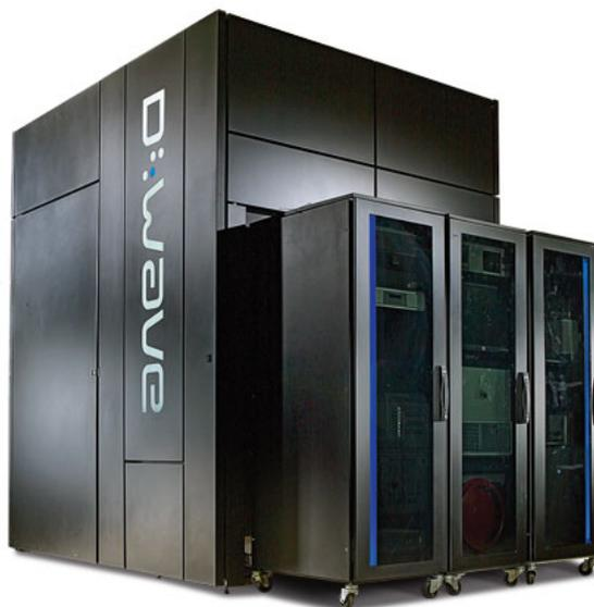
**Figure 1.5:** The D-Wave architecture is based on superconducting qubits. The first version was a 128-qubit processor, superseded in 2013 by a 512-qubit processor. Whether this quantum annealer outperforms classical computers is source of debate.
