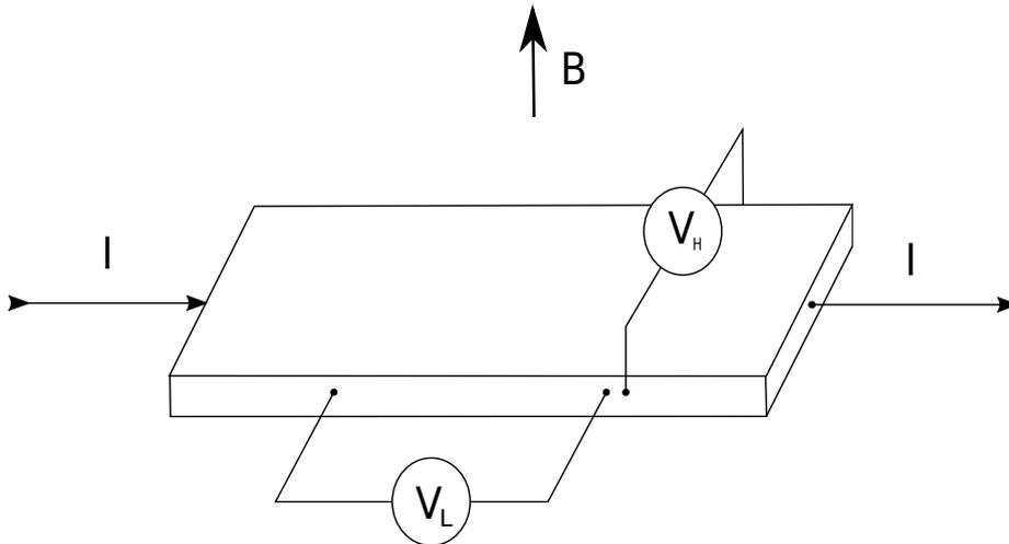
Figure 1.1: Sketch of a diagram of the classical apparatus used in Hall effect experiments.  $I$ ,  $V_L$ , and  $V_H$  are the current, longitudinal voltage and the Hall voltage, respectively. The longitudinal and Hall resistances are defined as  $R_L = V_L/I$  and  $R_H = V_H/I$ .
