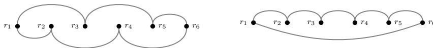
Figure 3.4: Optimal solutions for N = 6 , for the p > 1 (left) and 0 < p < 1 (right) cases. Notice how, in the 0 < p < 1 case, when all the arcs are drawn in the upper half-plane above the points than there is no crossing between the arcs.
